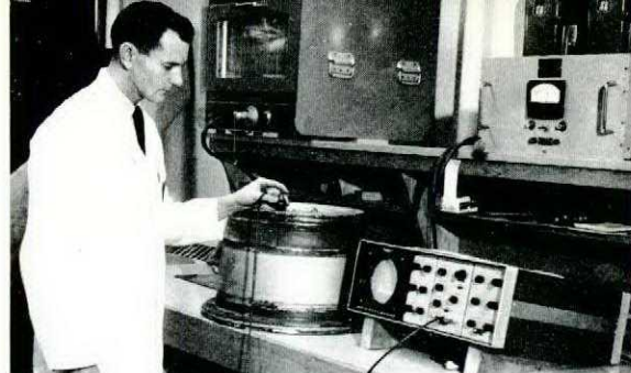
Operating ultrasonic reflectoscope on Yukon wheels to evaluate techniques for finding defects. Later, wheels will be ultrasonically checked in-situ on the aircraft.
