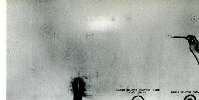
Port side of fuselage was pocked in several places
