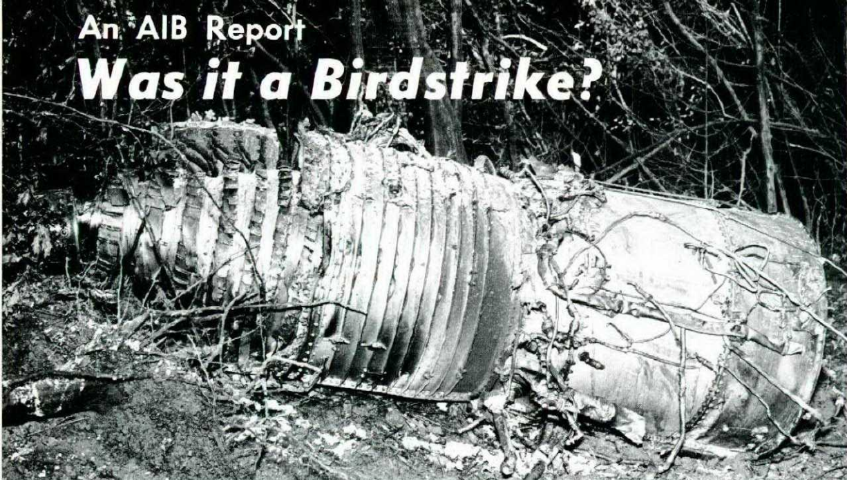
Tell-tale signs of bird ingestion appeared in several areas of the engine:
