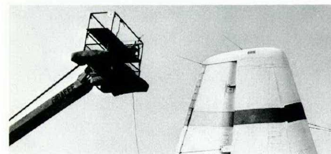
An Argus tail ready for X-ray exposure. The X-ray source is in the giraffe, and is aimed at an area where film is taped to the skin.
