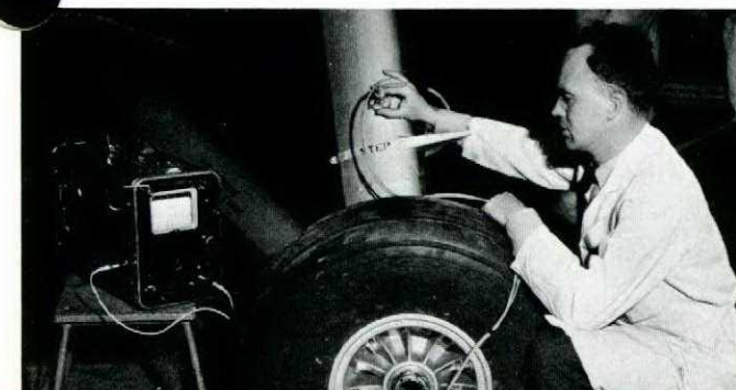
An Otter strut is mapped during the development of an ultrasonics inspection procedure. The equipment response in each area is recorded for comparison later suspect struts.
