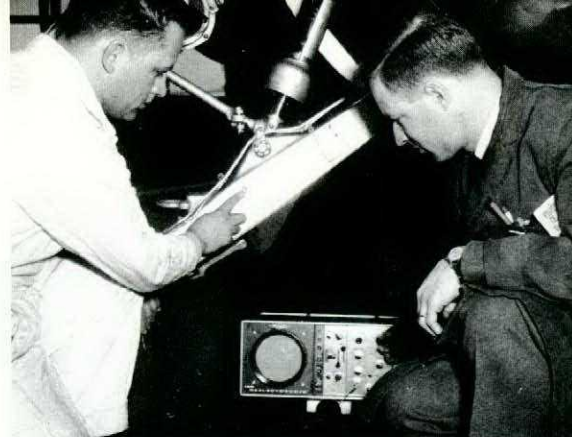
A CF104 main landing gear forging is inspected by ultrasonics.
