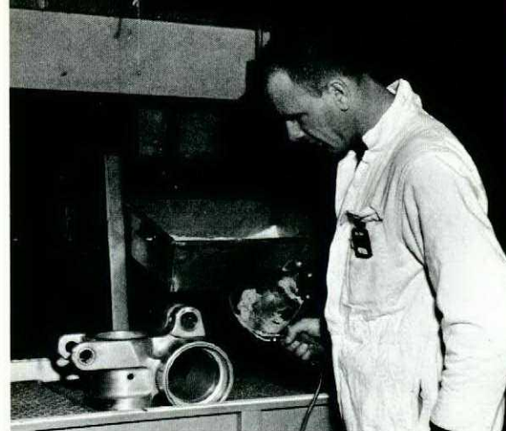
Dye penetrant inspection of a section of the housing of an Argus nosewheel gear.
