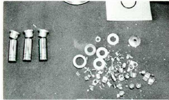
Hydraulic pump failure – the aftermath.
