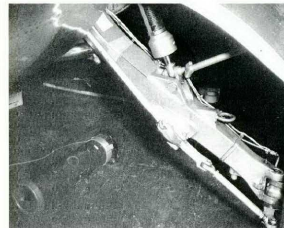
CF104 main landing gear forging is X-rayed. The film envelope is taped to the gear; the radiation source is below.
