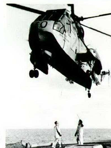
Sitting astride the Beartrap the Sea King has just completed the hauldown landing.
