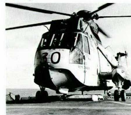
Sitting astride the Beartrap the Sea King has just completed the hauldown landing.
