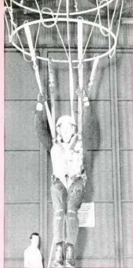
Each pilot is suspended in this rig to learn how to maneuver the parachute.
