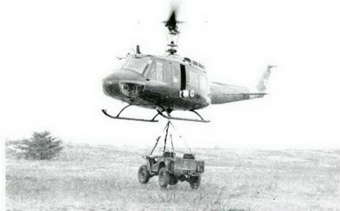
Until the load is well clear of the ground, the crewman monitors the lift-off.
