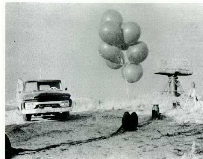
Bird carcasses are carried aloft to determine the radar reflectivity of various species.
