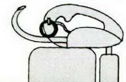
Aim nozzle (horn); remove pin; squeeze handgrip or trigger
