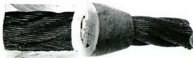
Note how properly swaged joint has cable wire embedded into sleeve.
