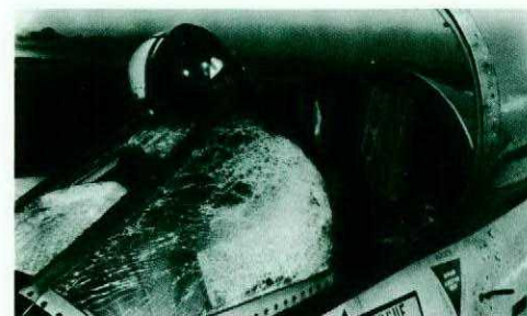
A two-pound bird struck at 420 knots exerts an impact force of 70,000 lbs.
