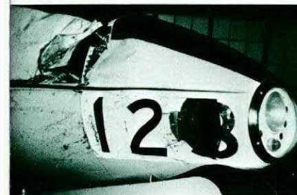
Ruptured CF104 tip tank.
