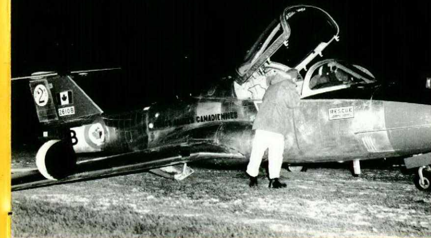
After a rain-saturated RON, the flight to colder climes ended with a maingear uplock jammed by ice.
