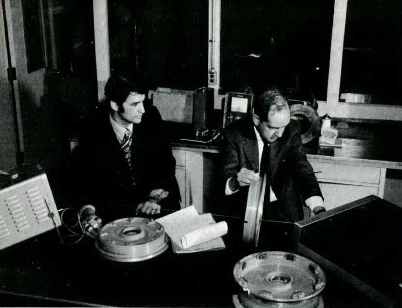
Evaluating the potential of eddy current or ultrasonic inspection of defective wheels.
