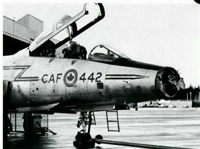
Battered Voodoo radome - the result of a lightning strike.
