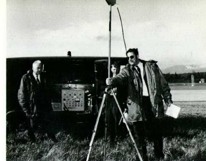
A QETE team performs an R.F. field strength survey at CFB COMOX. Calibrated test equipment accompanied the team in this airlift operation.
