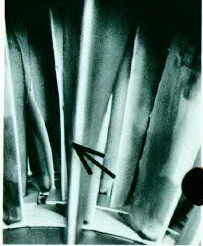
What: A drop tank pin How: The pin was snatched from a technician's hand by the right engine of a Voodoo running at idle power.
