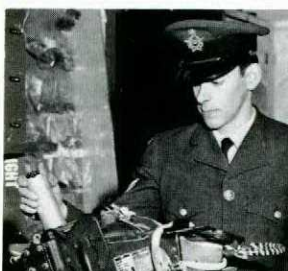
Four pound steel bar with markings of the United States Army Air Force may have been lying loose among the aileron cables for 25 years.
