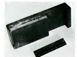
Four pound steel bar with markings of the United States Army Air Force may have been lying loose among the aileron cables for 25 years.
