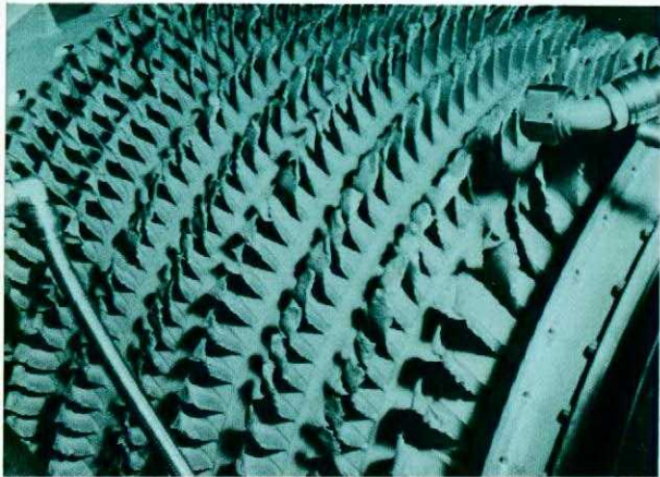
What: A punch How: Left in a CF104 engine area by someone, it was subsequently ingested.
