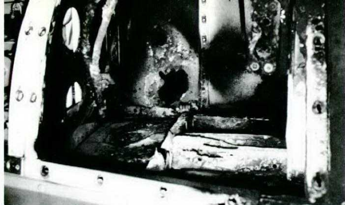
Batteries are usually considered harmless, but when mistreated they can react violently. This aircraft battery compartment shows the extent of damage caused by a Nickel-Cadmium battery failure.
