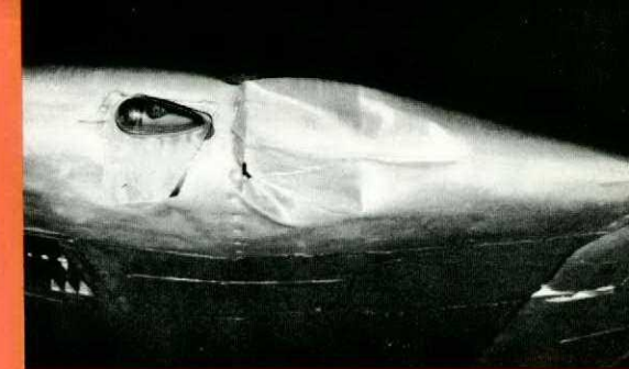
Slippery, ice covered tarmac and poor judgement by a towing crew resulted in the Cosmo wing crunching into a hangar door. The aircraft had been pulled out to allow the removal of another aircraft. Apparently the crew felt that since it cleared the doors on the way out, it should clear them on the way back in, an assumption that has embarrassed many towing crews in the past - during all seasons.
