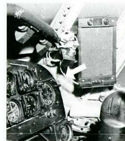
Correct cable routing for co-pilot's letdown holder - cable behind switch bracket.
