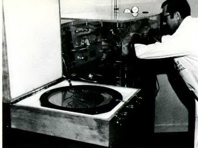
A precision pressure gauge being calibrated in the Applied Physics Lab by IE tech, Cpl. G. Cusson, prior to shipment to AMDU as a working standard.
