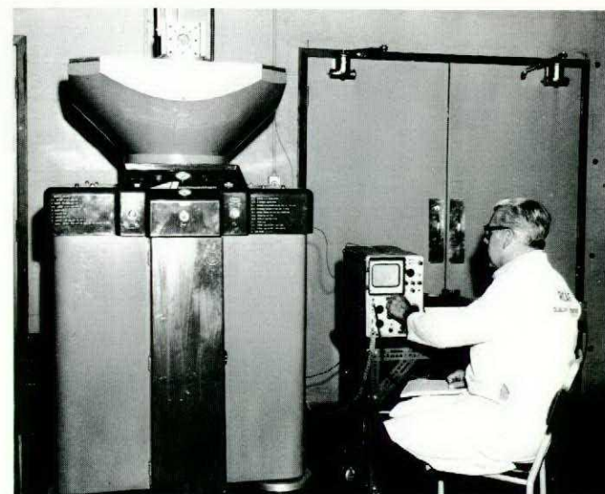
Specified-pulse shock machine investigating impact resistance of airborne instrument to withstand hard landings and excessive "g" forces.
