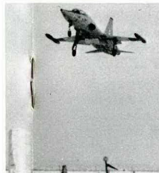
Figure 5. When there is a downslope in the approach zone, the pilot will believe the aircraft to be on a low, flat approach, assuming the slope is not readily discernible.
