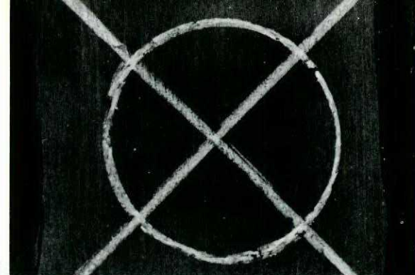
Photo 1 Alodized Panel - Grease Pencil - 20 hrs exposure showing no localized and minimal general corrosion.
