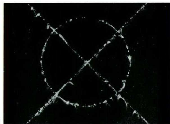
Photo 3 Alodized Panel - Graphite Pencil - 64 hrs exposure showing more severe localized corrosion and minimal general corrosion.
