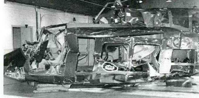
Fuel system integrity was maintained despite major airframe damage.
