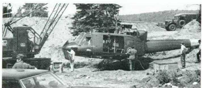
Investigators draining the fuel from a crashed CUH-1N.
