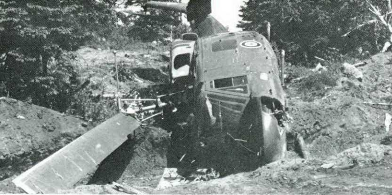
Fuel system integrity was maintained despite major airframe damage.
