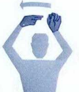
DISCONNECT GROUND ELECTRICAL POWER SUPPLY
