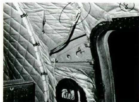
The problem has been corrected by attaching the escape rope to the aircraft structure above the swing arm assembly.
