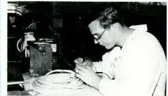
In the I & E section Cpl Hollett checks continuity on a CH135 wiring harness
