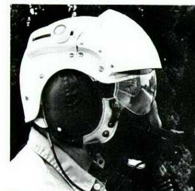
Photo 3 Correct size side view – DH 41-2 Jet helmet
