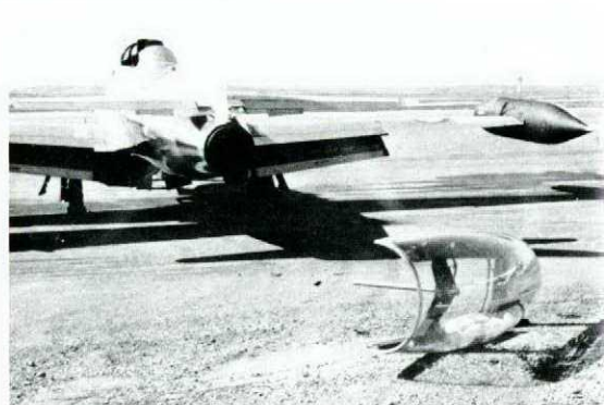
jettison handle was pulled on a T33 in Vancouver. This time however the pins were installed.
