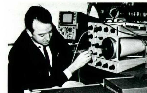
OSCILLOSCOPE PERFORMANCE IS MONITORED. MCpl A Cawston of the Calibration Centre monitoring the performance of a Cathode Ray Oscilloscope. The Cal Centre proves the performance of over 4,000 items yearly for the Canadian Forces and other government agencies.
