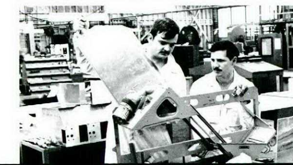
PRODUCTION OF PROTOTYPES. Cpl P Jobin of the metal shop checks the fitment of identification equipment in the holding rack from a high performance aircraft. Pte J Martin also of the metal shop checks the sliding fitment of rails.
