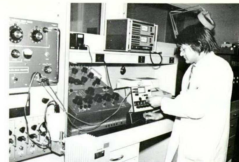
RF power is certified traceable to the National Research Council by Ray Tuokko using portable QETE standards.
