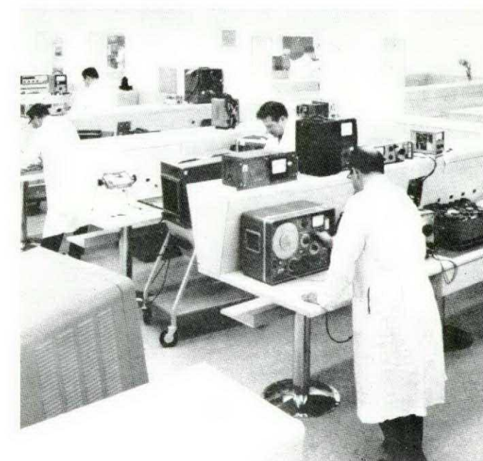
CAE contractor technician Walter Sametz verifying frequency and power of users signal generator.
