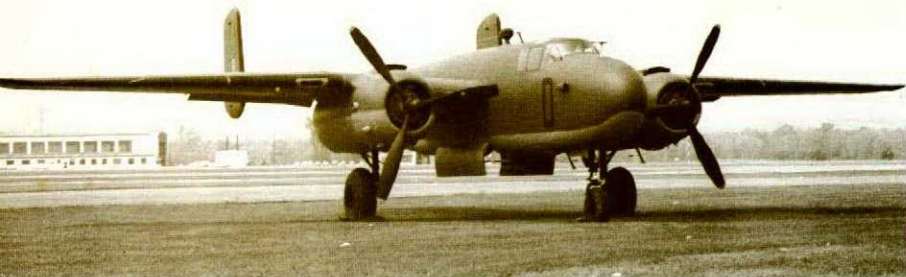
National Aeronautical Collection example of "hard nosed" Mitchell. This nose was sometimes modified to provide for the mounting of eight forward firing fifty calibre machine guns. American Units in the South Pacific mounted a 75 millimetre cannon in some aircraft used in the anti shipping role. Apparently it was quite impressive in effect.
