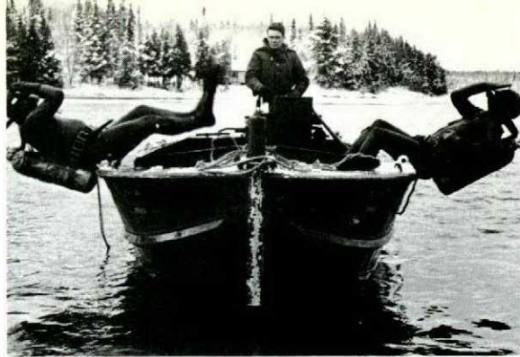
Divers of No. 1 Field Squadron enter the water using standard procedures. In addition to rubber rafts, the diving teams used this 19 foot inboard Boat Bridge Erection (BBE) most effectively during the operation. Besides acting as a diving tender it was used extensively to transport wreckage, including a heavy turbine section which had to be towed to the shore.
