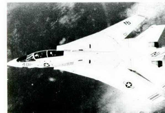
NFA - F-14, TOMCAT, utilizes Composite materials in the horizontal stabilizer
