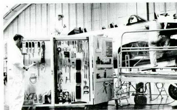
Tool board in use on the CFT-33 aircraft in the Repair section. Left-to-right: Cpl Ken Johnson, Pte John Belanger
