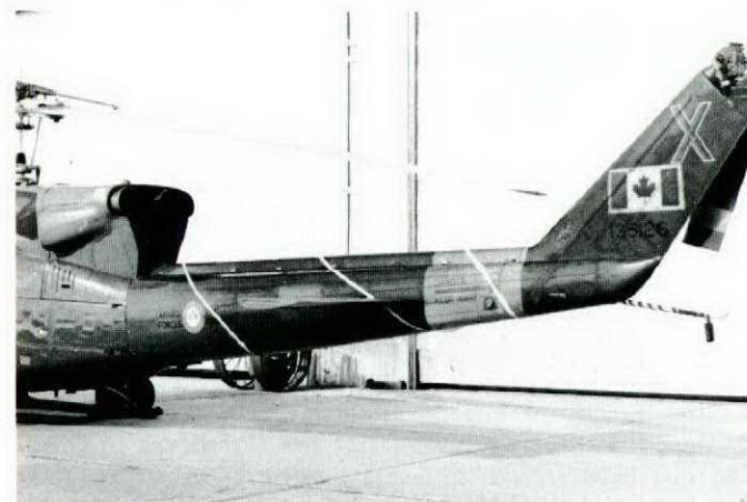
Masking Tape marks rotor cut points on tailboom.
