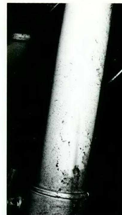
Split on actuator before cleaning.
