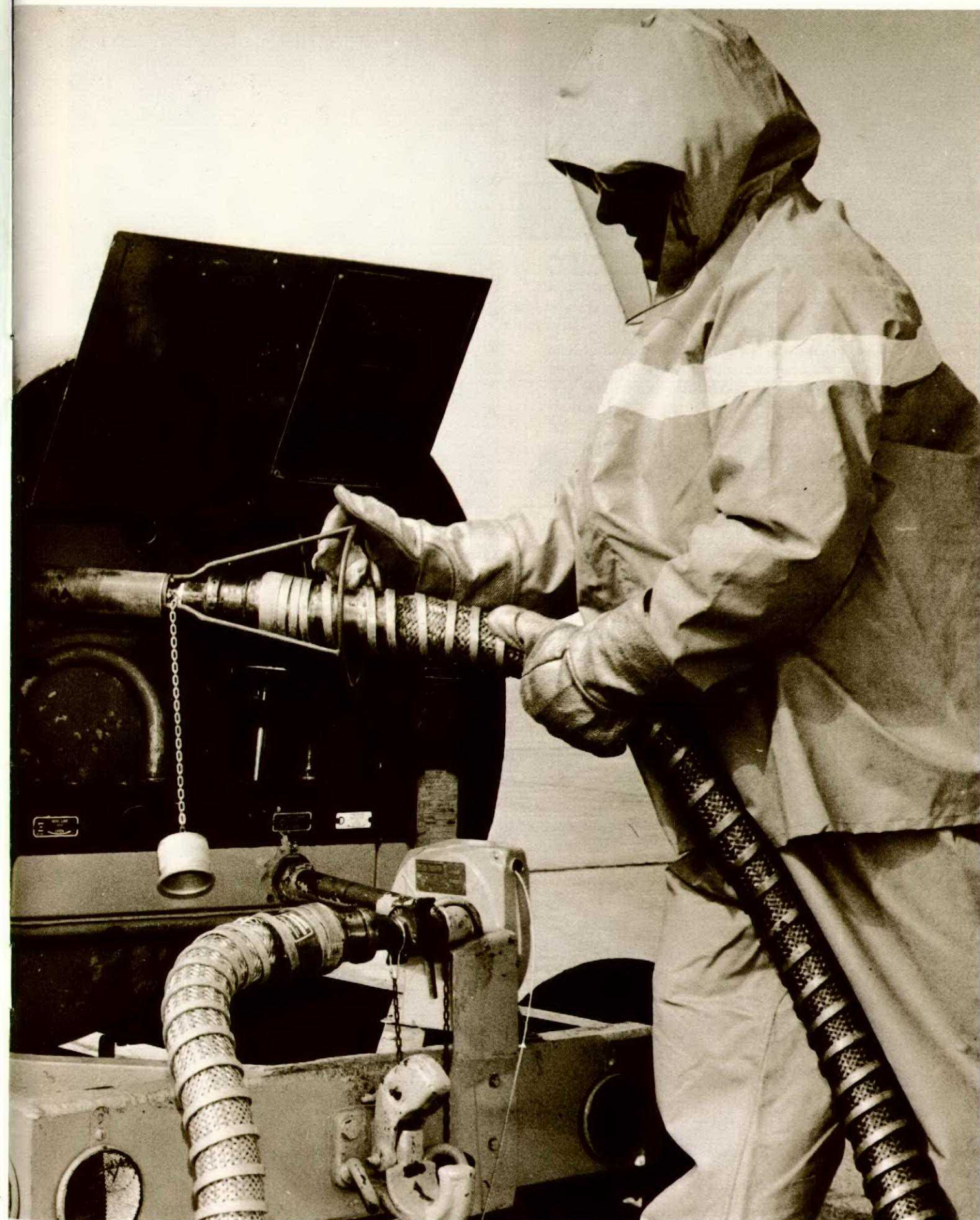
To replace the present LOX Handlers suit this outfit of lightweight neoprene and includes an attached hood and integral suspenders for the trousers. Reflective tape is put on the garment during manufacture.
