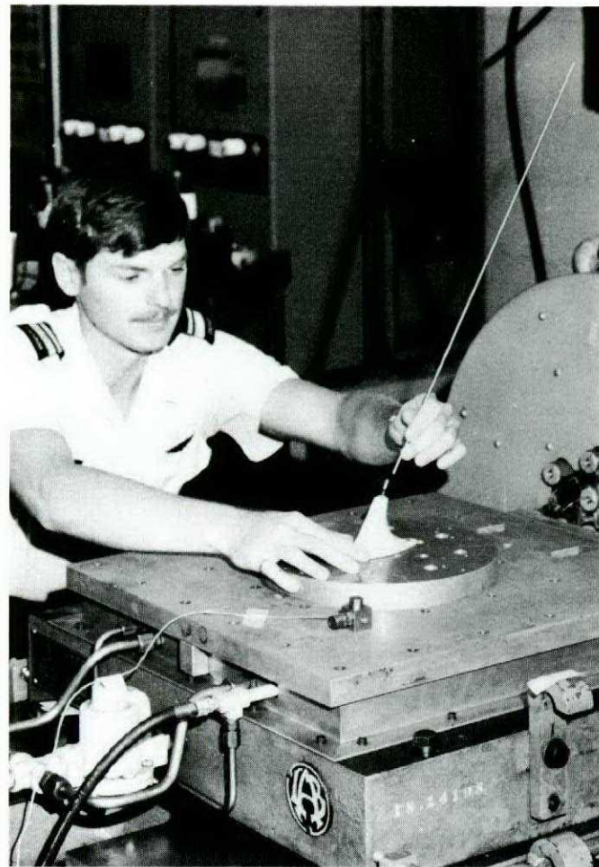
FIG 10. Failed DF 88 antenna after laboratory testing on the U.D. vibration machine 89B simulating actual service conditions.
