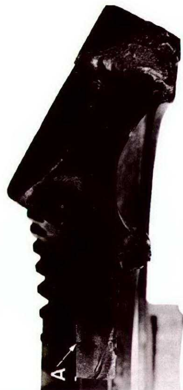
FIG 4. Spiral bevel combining gear fracture face showing classic fatigue features, crack origin at 'A'.
