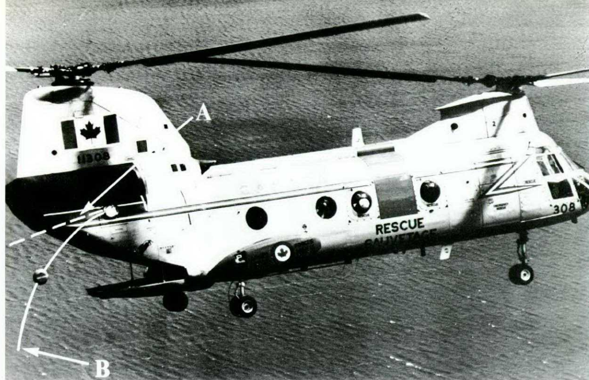
(A) Computed flight path and (B) Actual flight path of CPI during test release
