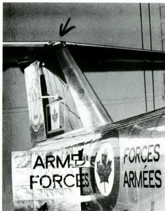
TUTOR — hail damage
