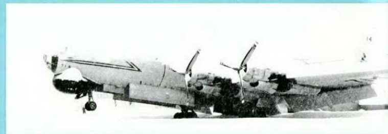
Lack of adequate weather warning and response procedures allowed snow to accumulate on the upper surfaces of this Argus during an unexpected snowstorm.
