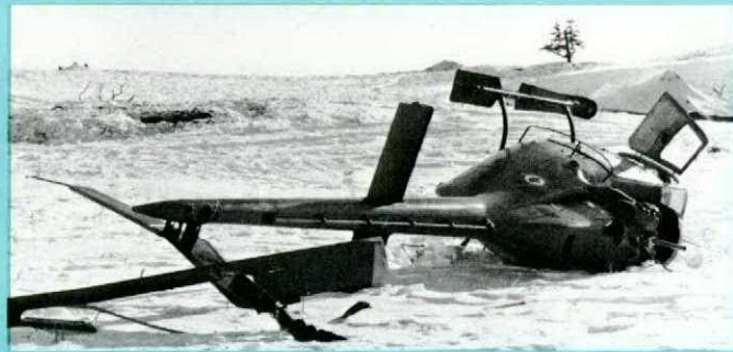
The pilot of this Kiowa failed to ensure that the skis were clear of snow / crust restrictions prior to take-off.
