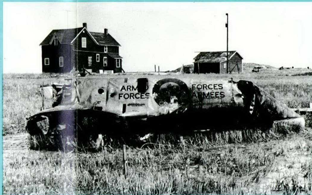
Ice ingestion is suspected to have caused engine failure of this Tutor.
