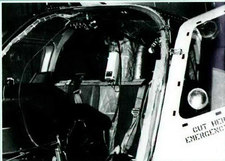
What happens when a Snow Goose attacks a Kiowa at 500 feet AGL and 100 KIAS (no, noise and rotor downwash did nothing to deter the assault).
