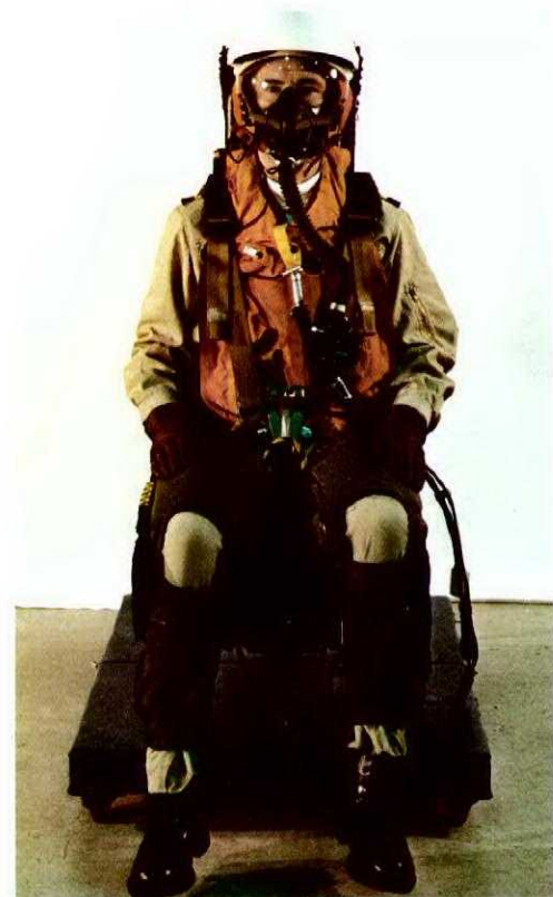
Simplified Combined Harness (SCH) with harness mounted oxygen regulator, life preserver, and anti-g coveralls. Note leg restraint lines.
