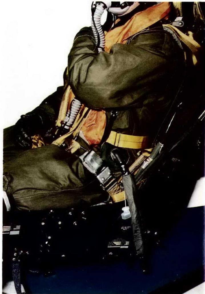
CF18 Seat Occupant Wearing the Integrated G-Suit/CF Constant Wear Immersion Suit
