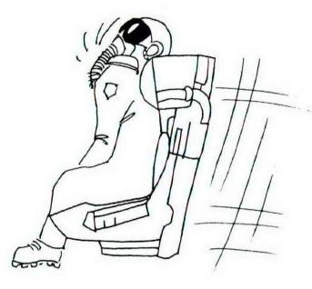
**Ouch!** You hit the windblast. At this stage, you are still travelling at the same speed as the aircraft. The windblast throws you back into the seat, extending your body up and back against the straps and seat! Your head should go neatly into the centre of the padded headbox but, if you are tumbling, it could hit the comer of the headbox or miss altogether. Some people lose consciousness at this stage.
