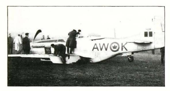
The pilot reports he made a normal selection for lowering the undercarriage and did not know that the wheels had failed to go down. The tower warned the pilot of the position of his undercarriage too late to avoid a wheels-up landing. Retraction tests carried out on the aircraft showed that although the undercarriage warning horn was unserviceable, the undercarriage warning lights operated normally.
