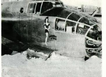
craft was parked a short distance in front of him, the pilot shut off the engines and managed to turn the aircraft into a snowbank by use of rudder. The resultant damage constituted a "C" category crash.
