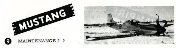
This pilot was carrying out an "air to ground" firing exercise when the engine began to backfire and a loss of power was experienced. Every possible attempt was made to clear the engine without results. The pilot then notified the control tower of his predicament and carried out a forced landing. The resultant damage to the aircraft constituted a "B" category crash but the pilot was uninjured.
