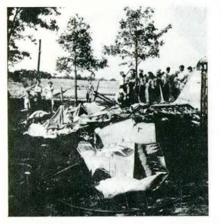
The direct cause of the accident is considered to be loss of control through over-controlling, after recovery from a spin at low altitude.
