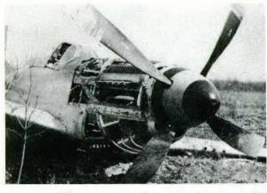
The port undercarriage collapsed and the wing tip dug in, causing a groundloop and subsequent damage to the propeller and fuselage.
