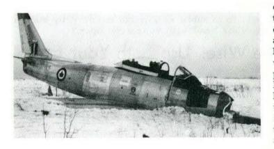
During the take off run, the pilot attempted to ease the control column back at an airspeed of 110 knots and found that it was necessary to apply pressure with both hands. As the aircraft had, at this time, used up most of the runway, it became apparent that he would not get airborne in time. The pilot cut the throttle and applied full brake.
