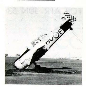
The pilot made a flapless wheel landing under crosswind conditions. As the tail of the Harvard lowered it swung to the right. The pilot overcorrected and then appeared to lose control. The aircraft zig zagged down the runway until it eventually ran off the side into the soft infield and flipped upon its nose. The cause of this accident has been assessed "Pilot Error".
