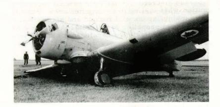
After making a wheel landing the "Hazard" swung to starboard. The pilot overcorrected and the aircraft swung to port. Along with his overcorrection the pilot applied full power. The result is obvious. A vicious swing to port which the pilot could not overcome. Considerable replacement damage resulted.
