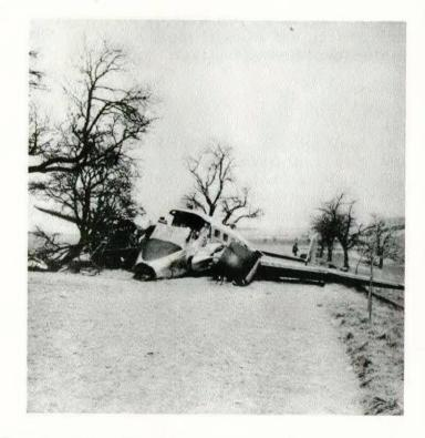
jured, three of them seriously. The aircraft was extensively damaged. The cause of the double engine failure was determined to be water in the fuel. An investigation is now under way to determine the source of the water found in the fuel. It has been recommended that all RCAF refuelling tenders have water strippers installed.
