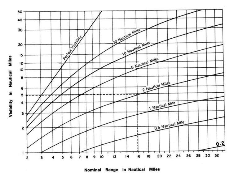
The light list in column 7 gives the nominal range of each lightstation optic where there is sufficient light to be seem 2 nautical miles or more when the meteorological visibility is 10 nautical miles.
