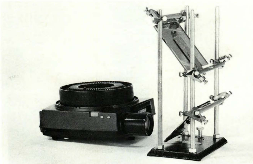
Fig. 4. Projector and framework for mirrors, showing bolt to adjust level and screws to adjust inclination of mirrors.
