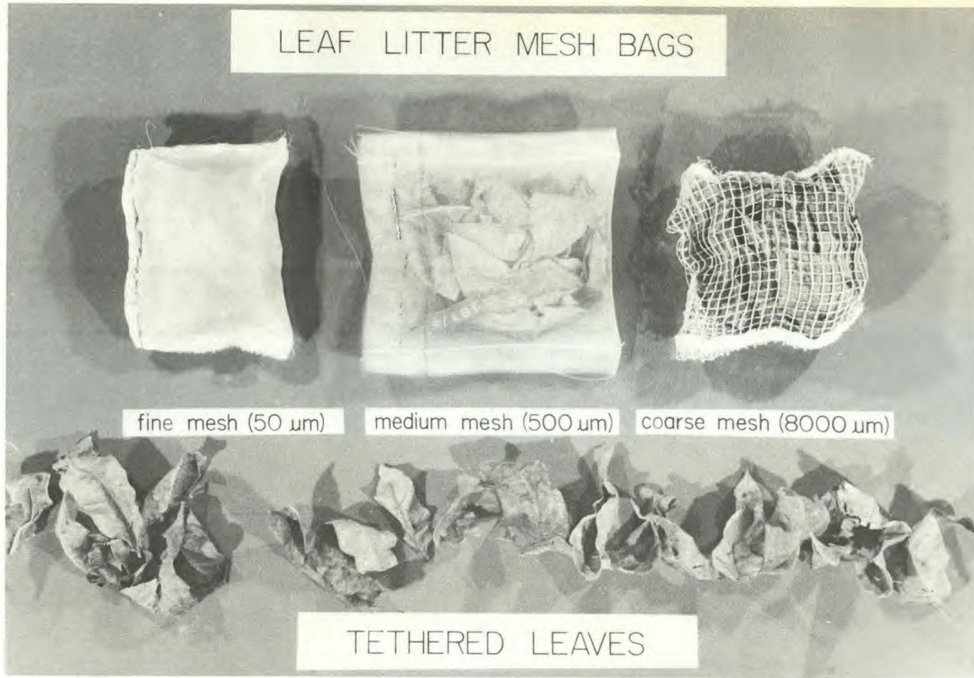
Fig. 5. Different sized mesh bags and tethered leaves used for leaf litter processing experiments.
