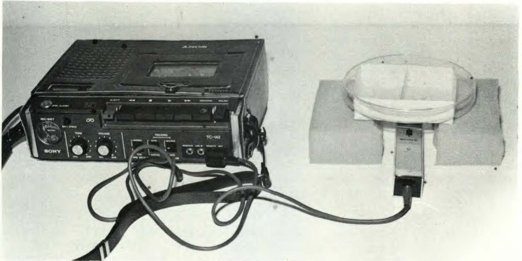
Fig. 10. Drumming chamber and recording apparatus.
