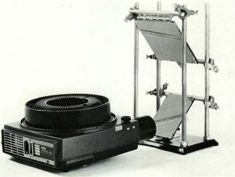
Fig. 3. Projector and framework for mirrors to rectify inverted images (piano hinge suspending top mirror clearly visible).
