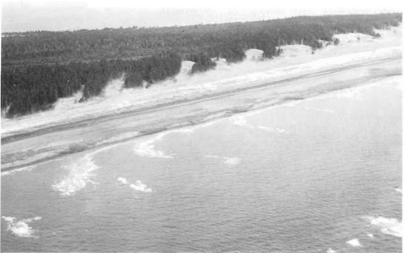
FIG. 8.11. Modified rip cells (horizontal circulation cells) near Rose Spit, Queen Charlotte Islands, July 1979. Rhythmically spaced cells caused by waves breaking over bars that project from shoreline; circulation pattern is shoreward flow along transverse bars and seaward rip current mid-way between bars. Large dunes in background over 10 m high and driven into forest by strong southeasterly gales. (Courtesy J. Harper)
