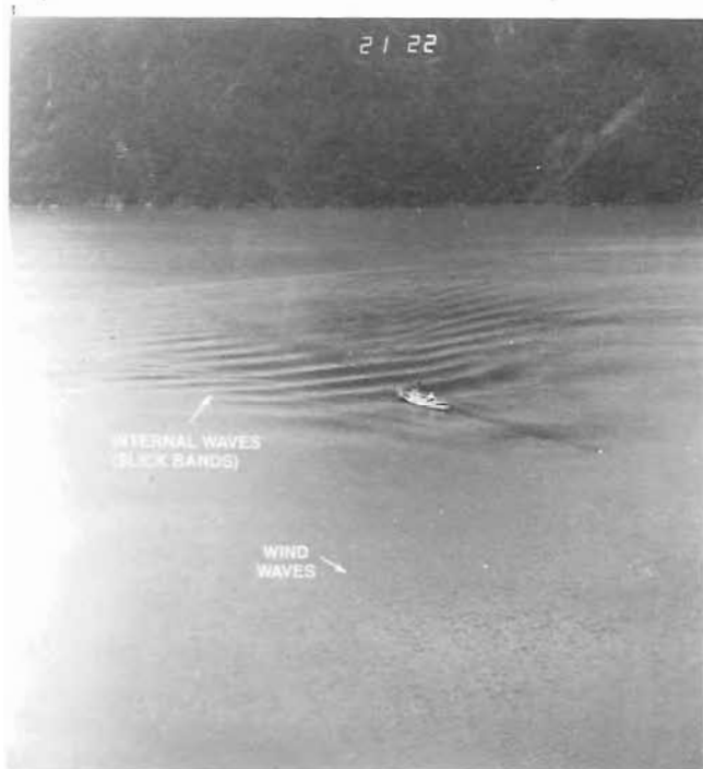
FIG. 6.24. Surface slicks in Orford Bay, Bute Inlet, associated with a group of ship-generated internal gravity waves (an internal wake), July 1972. RV Endeavour (draught, 3.7 m; length, 65.0 m), generated internal waves by streaming astern along a fixed track, adjusting engine power to obtain maximum "dead water" effect. The resulting wave group, formed at interface of 4-m thick surface brackish layer and deep saline water beneath, was studied by reversing ship direction and transversing waves. (From Hughes and Grant 1978)
