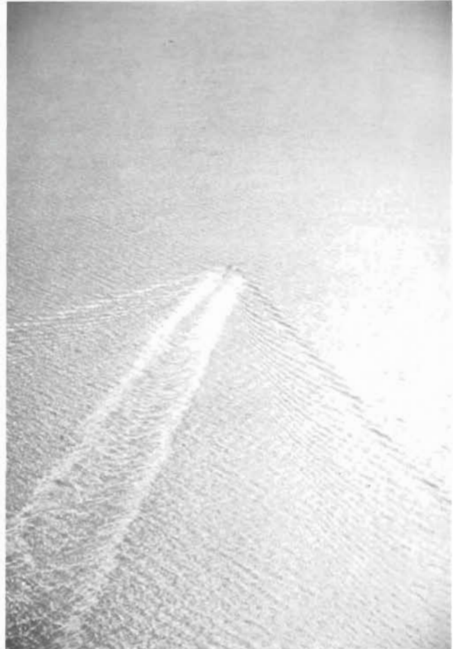
FIG. 6.27. Ship-wave pattern generated by submarine in Strait of Georgia. Wake dominated by long waves with crests nearly perpendicular to path of vessel. Two diverging wave systems visible with angles in wedge-shape wake roughly equal to 140^\circ . (Photo by author)
