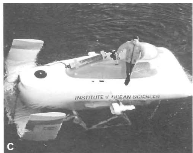
FIG. 1.16. Research vessels of the Institute of Ocean Sciences, Patricia Bay, B.C. (A) Canadian Scientific Ship (CSS) Parizeau , displacement 1929 t, length 64.3 m; (B) CSS Vector , displacement 505 t, length 39.6 m; (C) Pisces IV submersible, length 6.1 m, maximum depth 1800 m. (Submersible photo courtesy C. MacKay; ship photographs by author)
