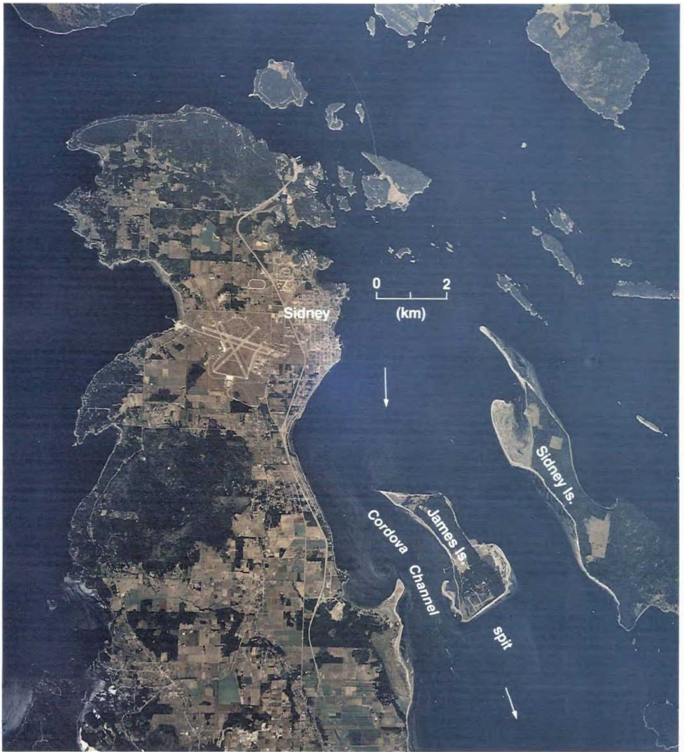
PLATE 11. James Island, southeast of Sidney, Vancouver Island. Two light-colored, wavelike trails (presumably suspended bottom sediments) appear to have formed in the lee of the island at the sides of James Spit as the southward flowing ebb current separates from the end of the island. (Photo also shows Sidney Spit at the northern end of Sidney Island; see Fig. 2.26d.). (Government of British Columbia Air Photo, August 1972.)
