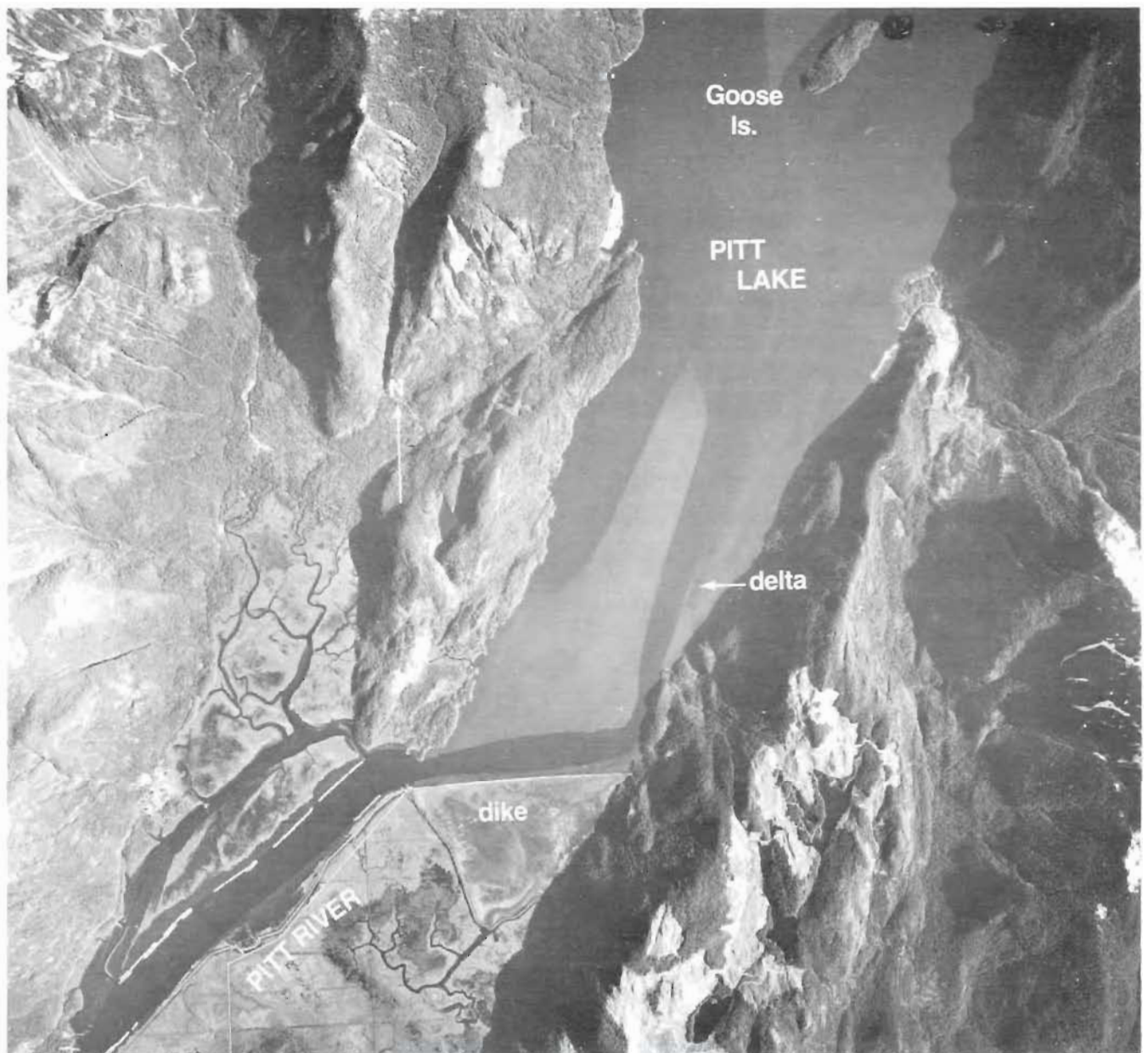
FIG. 10.30. Aerial photograph of lower Pitt system. Delta formed at south end of Pitt Lake by upstream movement of Fraser River sediments along Pitt River to lake. Pitt tidal delta has advanced 6 km into lake in last 4700 yr, average rate 1.28 m/yr. (Ashley 1977; British Columbia Government Photo 1954.)
