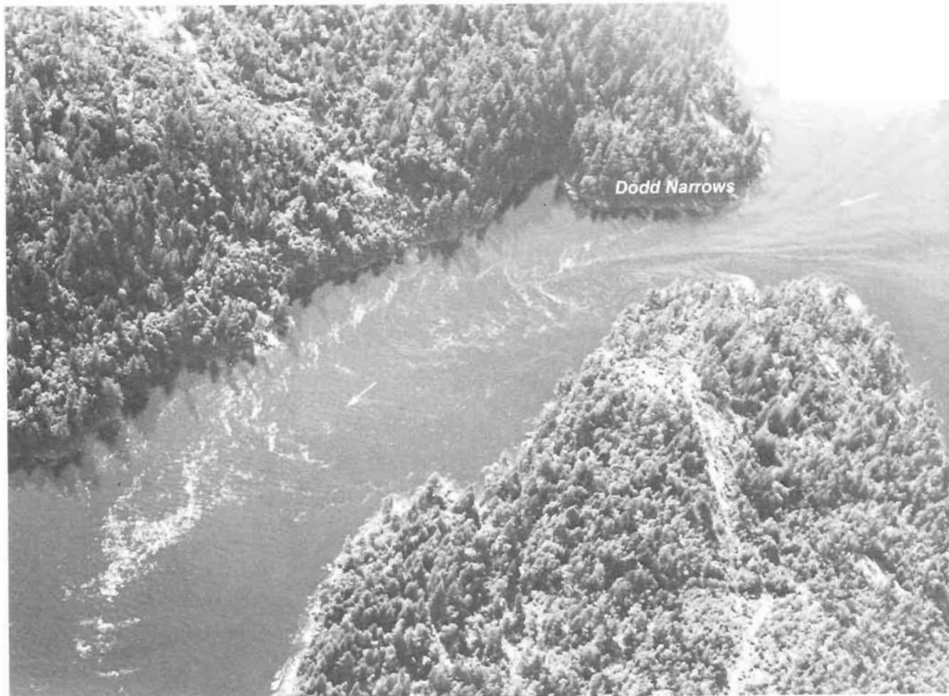
FIG. 4.9. Strong ebb current flow southward through Dodd Narrows from Northumberland Channel near Nanaimo, Aug. 13, 1962. Flow is relatively laminar (smooth) through neck of narrows but becomes turbulent in broader basin to south. (Courtesy R. H. Herlinveaux)
