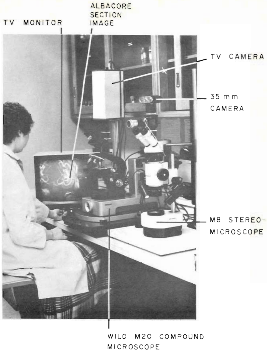
FIG. 15. Hitachi TV monitoring screen using a Wild M20 research microscope showing an albacore fin section. Also, a Wild M8 stereomicroscope set up for photomicroscopy.
