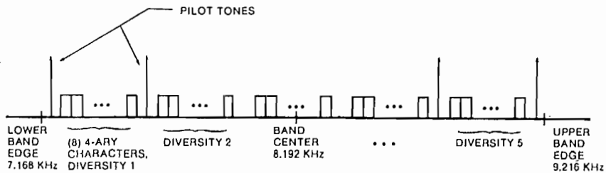
FIG.3: PILOT TONE AND DATA SPECTRAL ALLOCATIONS
