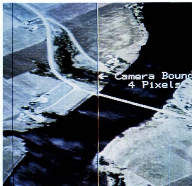
FIG. 34b. The same as in Fig. 34a but expanded by a factor of 2 about the cursor. The expanded area shows the effect of overlap and poor array performance near each edge.
