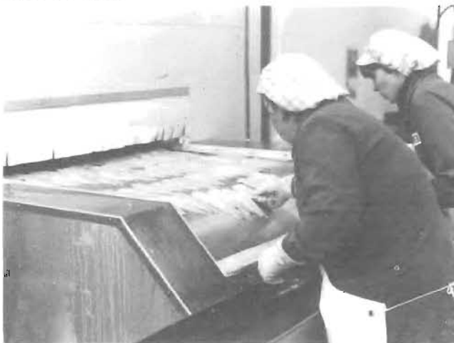
Fig. 3. The "Torry" continuous air blast freezer for IQF (Individually Quick Frozen) Products.
