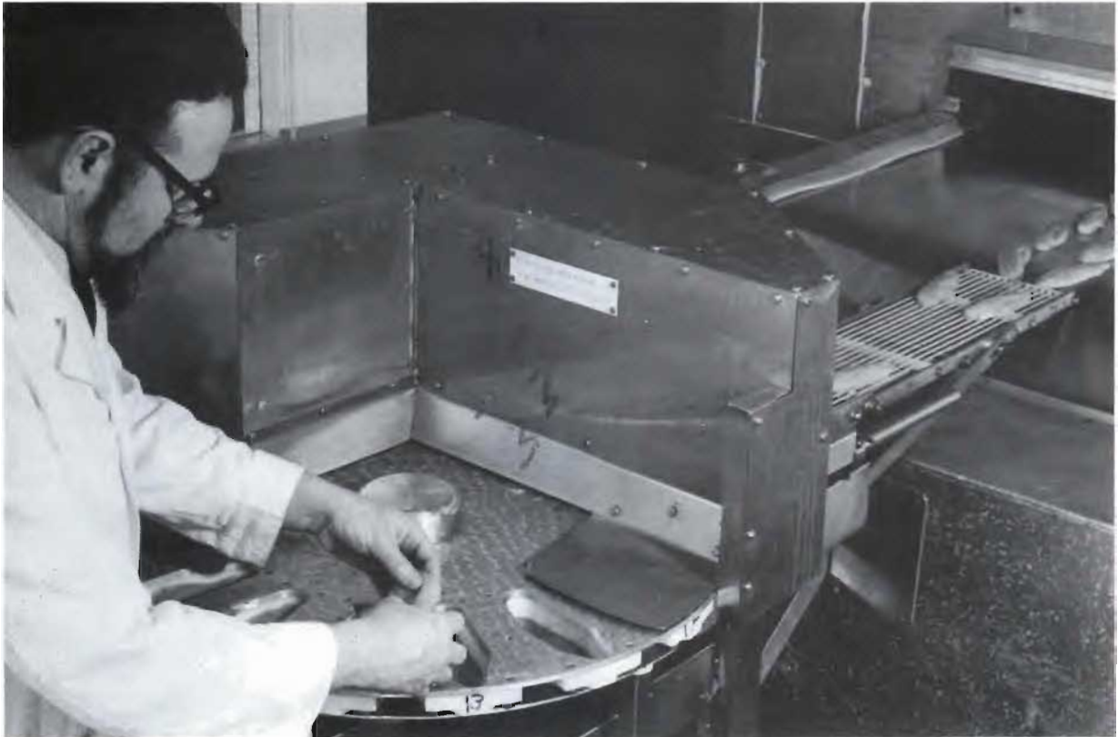
FIG. 1. The TRS (Torry Research Station's) prototype machine for forming composite fillets.
