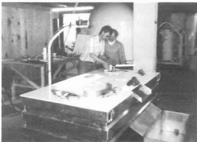
Specimen table — Fish are moved along a conveyor belt (circular in this case) for image assessment by an electronic camera (mounted on a metal arm and positioned directly above the conveyor). This data is then processed by algorithm to determine species, length, and weight.
