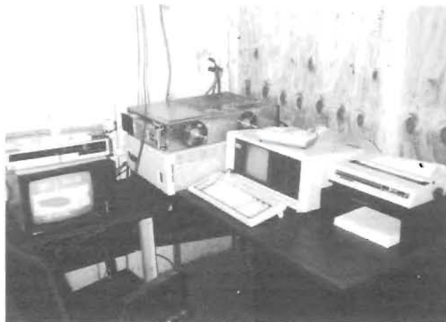
Onboard fish monitoring system — The complete EDP system includes a computer, camera, monitor, output terminals, and software.
