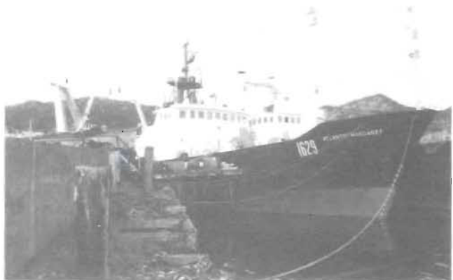
Atlantic Class stern trawler Atlantic Margaret , 153' LOA, owned and operated by FPI, undergoing refit and installation of the Contrawl System at the Burin Refit Centre in Newfoundland.
