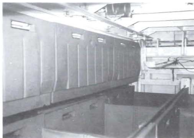
Forty-eight 480-litre boxes can be manipulated and stored in the forward hold of the Atlantic Margaret . This is done completely automatically after the containers leave the factory deck.
