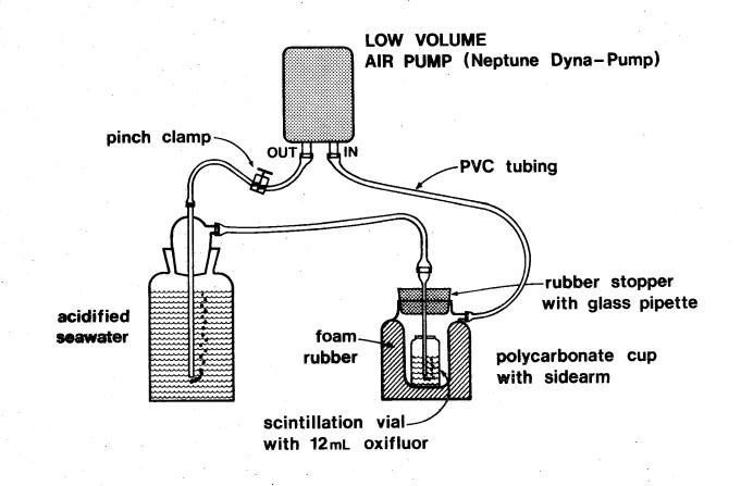
Nuclear) adsorbed the CO over a 10 min period (see figure). Bubbling rate was set by eye, so that bubbling did not cause the water to "boil" but still created steady mixing in the sample. (WJ & FAW)
