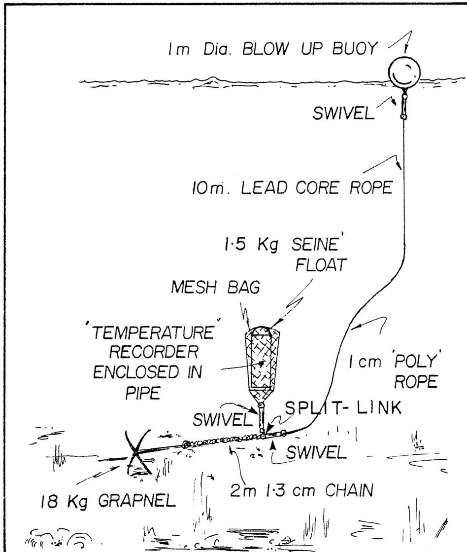
Mooring Diagram for Temperature Recorder
