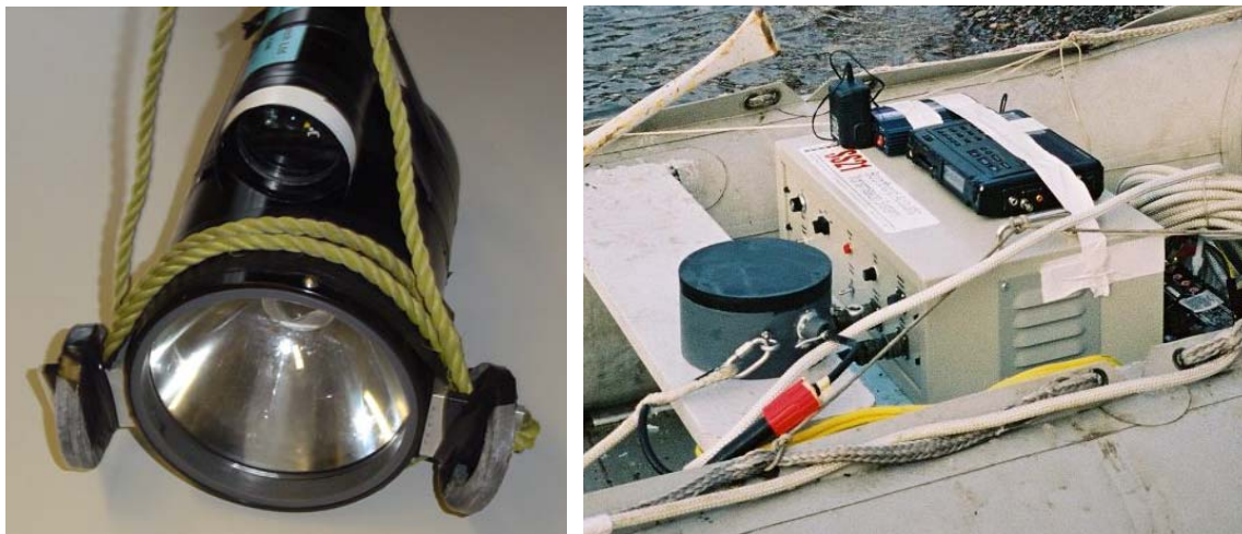
Figure 7: (Left) Underwater xenon strobe light with orientation monitoring unit mounted on top; (Right) Underwater acoustic source consisting of low-frequency piezoelectric transducer (on boat seat), power amplifier unit, and digital recorder for playback of pre-programmed waveforms.
