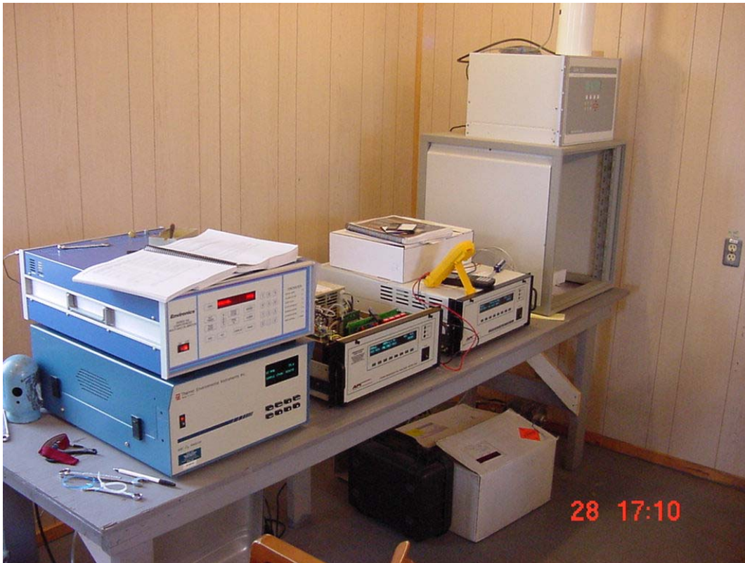
Figure 3: Calibration Equipment and Gas Analyzers at the Sable Island Station During a Service Session
